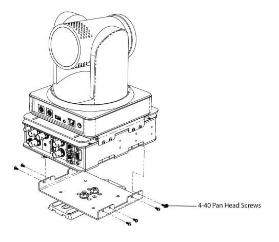
Figure D: Installing the PTZ camera on the VB enclosure
