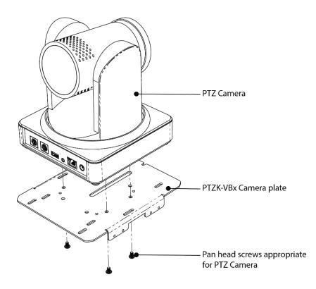
Figure A: Installing the camera plate on the PTZ camera
