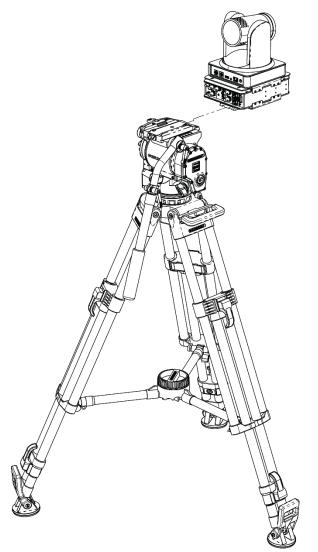
Figure E: Slide the PTZ/VB assembly on the tripod head
