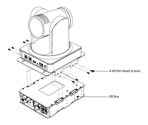
Figure C: Installing the PTZ camera on the VB enclosure
