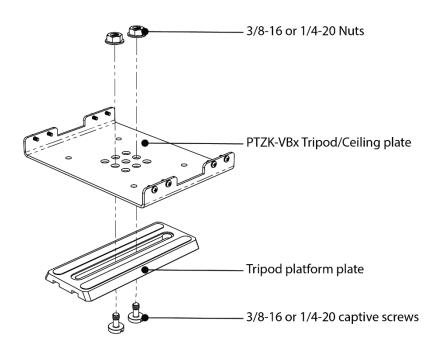
Figure B: Installing the platform plate on the PTZ camera
